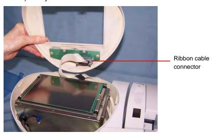
5. Open the clamps on the ribbon cable and disconnect the ribbon cable from the button control panel.
